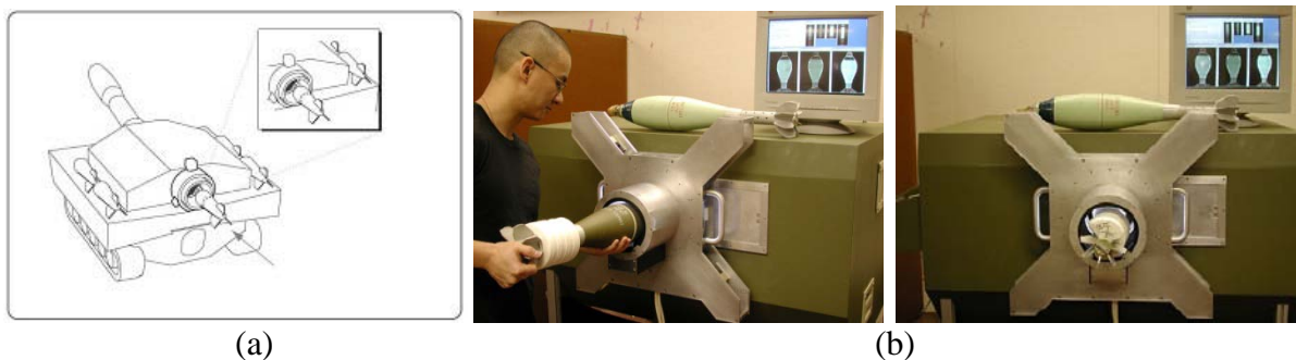
Figure 17. (a) Concept future force mortar with PIDS system inline with loading port; (b) PIDS identification and inspection system as implemented for port inline application
