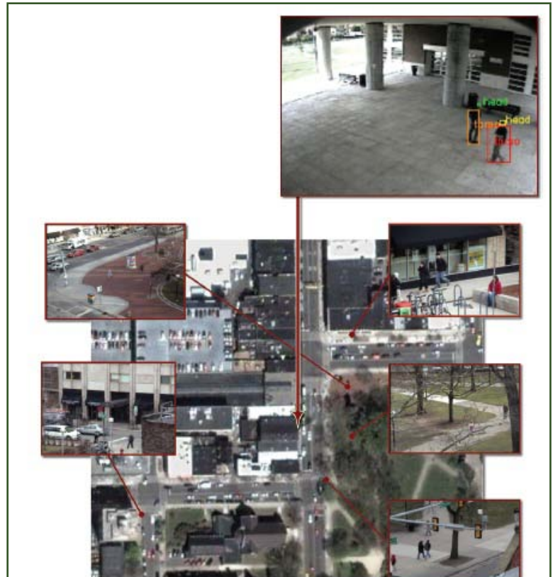
Figure 5. Applying human motion tracking and intention detection to video surveillance
