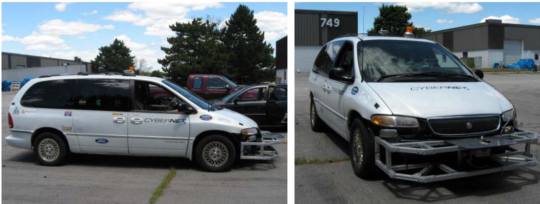
Figure 10. Cybernet Automated Minivan “Cybervan” ( www.cybernet.com/urbanchallenge ).
