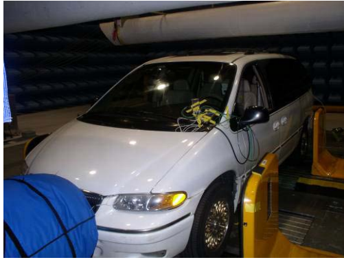
Figure 27. The Cybernet Grand Challenge Vehicle under test at the General Motors Electromagnetic Test Facility for determination of microwave weapon assault susceptibility (projects for the Dept. of Homeland Security and TSWG)
