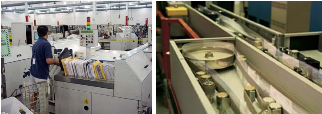
Figure 21. USPS letter and flats sorting machines using handwritten and machine print OCR automation developed by Cybernet staff while they worked at the Environmental Research Institute of Michigan, 1987-1990
